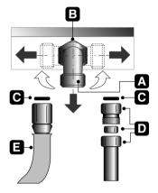
**Connection with flexible pipe:** use only flexible pipes conforming to standard regulations in force, inserting gasket **C** (supplied) between fitting **A** and flexible pipe **E**.
